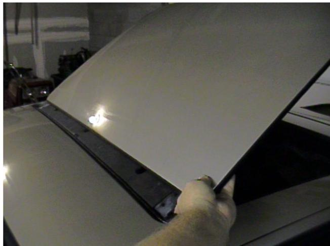
2. Lower the back of the sunroof in to the sunroof opening. It should sit flush with the top of the roof.
