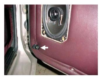
6. Pull out on the interior door handle as if you were opening the door. Behind the handle you'll find a Phillips head screw which must be removed. This is a rather awkward operation and caution should be used to prevent damaging the door handle.
