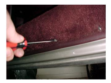
5. When the door pocket is removed, you'll find a plastic mounting block at the front of the door panel for the front door pocket screw. Using a Phillips screwdriver, remove the plastic mounting block.
