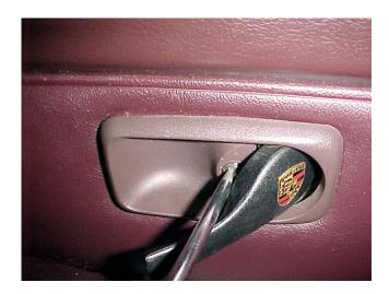
7. Using a Phillips head screwdriver, remove the three screws underneath the door arm rest. These screws are threaded into the door at approximately a 45° angle.
