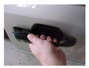
3. On the back side of the door handle you'll see a white plastic piece which is attached to a button on the door handle lock mechanism. Using a flat tip screwdriver, gently pry the white plastic piece off of the door handle.
