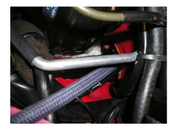
11. If the paper gasket is torn, replace it with new. Take care to ensure that you don't upset the angle pipe at the top of the clutch master cylinder. If it breaks or comes out of the clutch master cylinder body, you will be where I am, which is replacing the cylinder with a new OEM one.
