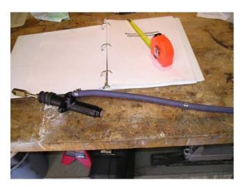
6. Install new clutch master cylinder with hose attached to firewall gasket. Have a friend guide the rod into place on the clutch pedal so it's not jammed up.
