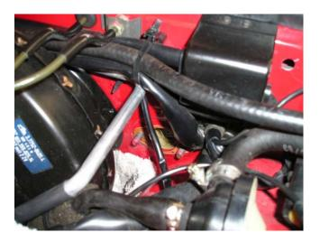
12. Using slip-joint pliers, gently pull the clutch master cylinder away from the firewall. Once clear of the studs, pull up at an angle to pull the entire clutch master cylinder, boot, connecting rod and clevis from the firewall. Bag the parts.
