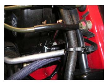
7. Install hard line to front of clutch master cylinder with 12mm-flare nut wrench. Have patience, as there is little room to work here.
