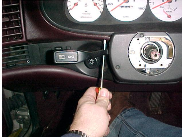
7. The vents in the center of the dash are an integral part of the trim piece surrounding the instrument cluster. There are several Phillips screws located in the vents which must be removed to remove the instrument cluster trim piece. There is one Phillips head screw located in the vent area to the far right of the instrument cluster. There are two more Phillips head screws located in the vent area closest to the instrument cluster. Remove all three of these screws.
