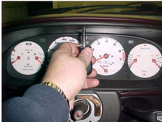
6. Remove the two Phillips head screws which thread into the plastic trim piece from the bottom on either side of the steering column.
