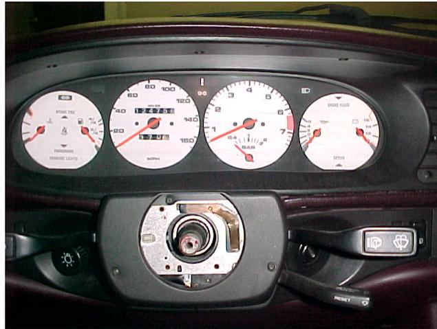
5. Remove the three Phillips head screws located in the top of the plastic trim piece around the gauge cluster. A stubby Phillips head screwdriver works well here.
