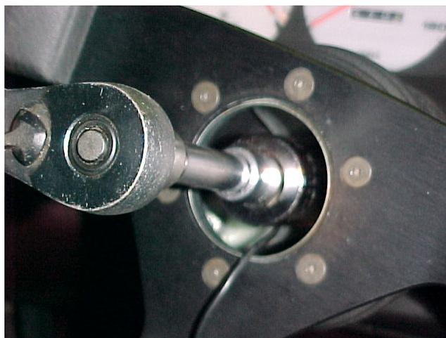
3. Using a scribe, paint pen, or nail polish, mark the orientation of the steering wheel to the end of the steering shaft. This will facilitate easier installation during re-assembly.
