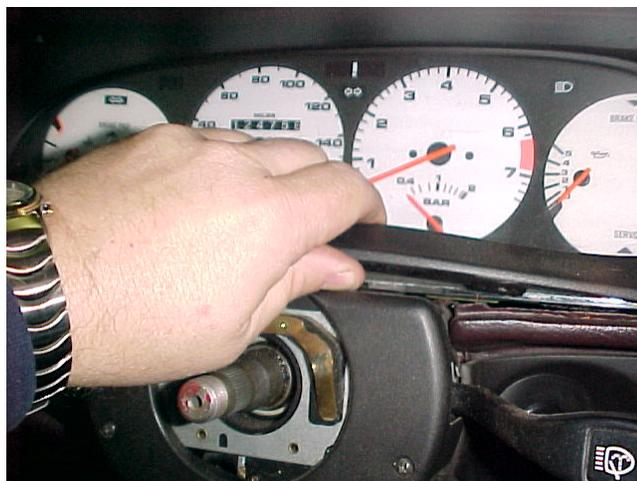
9. With the trim piece removed, you will now see the four Phillips head screws which hold the gauge cluster in the dash. Remove the screws and slide the cluster forward to access the electrical connectors on the back of the cluster.
