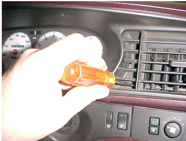
8. Lift up on the bottom edge of the trim piece right behind the steering column trim piece. This will allow the gauge cluster trim top of the steering column. You may also need to pull down slightly on the top of the trim piece to clear the dash. The instrument cluster trim piece should now slide out of the dash.
