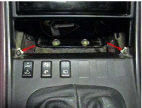
b. Remove the ash tray from the center console by pulling it straight up out of the console and remove the two Phillips head screws at the back of the console.
