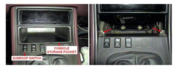
b. Remove the ash tray from the center console by pulling it straight up out of the console and remove the two Phillips head screws at the back of the console.
