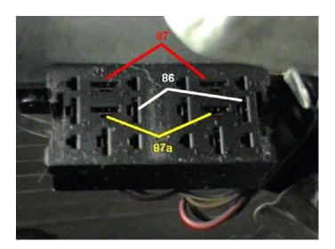
On early 944 sunroof systems, install the ignition key into the ignition (not required on later sunroof cars). With a multimeter, you should read 12 VDC on both terminal 87s to ground and less than 1 ohm resistance between the 86 terminals to ground and 87a terminals to ground. If the voltage reading on the 87 terminals is bad, check the following:
