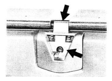
4. If the micro-switch is to be replaced, unsolder the wires from switch and install a new switch.
