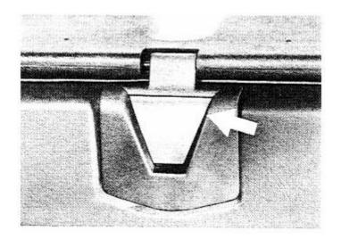
3. Once the flap is removed, use a Phillips head screwdriver to remove the retaining screw from the mount and press the mount off of the wind deflector bar.
