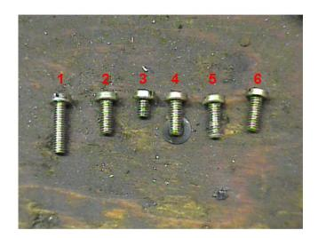
3. First remove the two screw that hold the relay block in place (one long, one short). Move the relay block out of the way and remove the screw underneath the block. Remove the remaining three screws.
