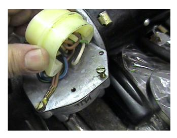
4. Remove the gear assembly cover carefully as there are electrical contacts on the back side of the cover. Be careful when you remove the cover as there is a small ball bearing in the center of the contact wheel. Remove that ball bearing and set it to one side so you don't lose it.
