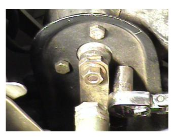
5. Lower the headlights back to the full down position. This is done to retain the motor-to-linkage alignment when the motor is removed.
