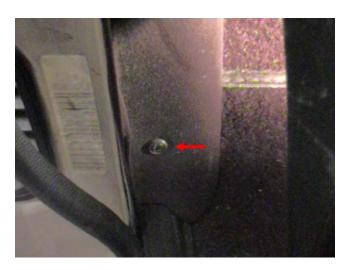
4. Remove the Phillips Head screw at the base of the trim panel below speaker opening.
