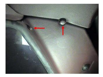
9. Use one of the following two options to loosen the interior panel covering from the window opening:
