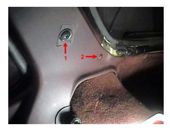
7. Remove the rubber cover from the rear seat latch pin. When you remove the cover, you'll see a hex shaped portion of the pin. Use an open end wrench to remove the latch pin.
