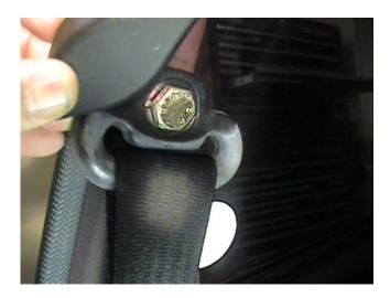
6. If your car is NOT equipped with rear shoulder harnesses, it will have a large Phillips Head screw in place of the shoulder harness mount. Remove this screw (1). Also, remove the small Phillips Head screw below and toward the rear of the car (2) from the shoulder harness mounting point.
