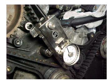
5. Push the tensioning roller against the cam belt until the locking pin on the tool engages. Read the tension on the dial.
