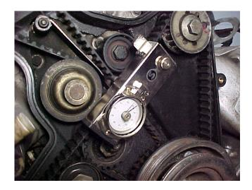
4. Adjust and recheck the belt until the tension is within the specified limits.
