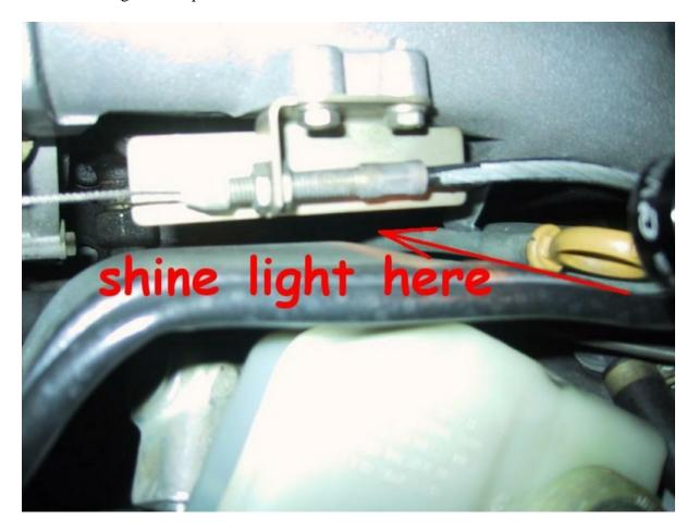
Then if you look at a 45-degree angle from the front towards the bottom of the dipstick, you should be able to clearly identify if the turbocharger has the 1" flat square. If it has the square, it's a K26-6. No square, it's a K26-8 (see picture of a K26-6 below).
