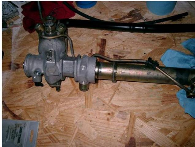
5. Remove rubber boot from the top of the control tower that surrounds the spindle, then remove the three 10mm bolts. You can then carefully pry the top off of the control tower. The top will have 1 wiper seal in it, and an o-ring as seen below. Note the orientation of the wiper seal before you remove it. The groove side will be on the inside of the tower, with the flat side pointing outward.
