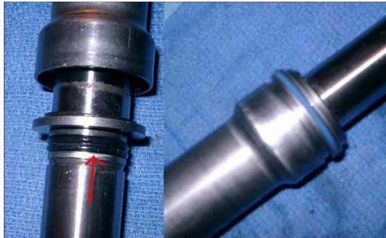
11. The shuttle. Remove the shuttle from the steering shaft. Inside is a wiper seal and a hard plastic spacer underneath it. Using the appropriate sized socket, pound the seal out of the shuttle, and install the new spacer and seal. Again the groove in the wiper seal will face out, or toward the passenger side of the vehicle.
