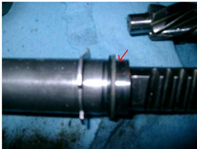
13. The bronze steering sleeve. Inside is a wiper seal, a plastic spacer, and a plastic guide ring. The plastic guide ring is removed first, using a small pick and needle nose pliers. When I removed it, I thought I was going to break it, but it seemed to flex pretty easily and come out.
