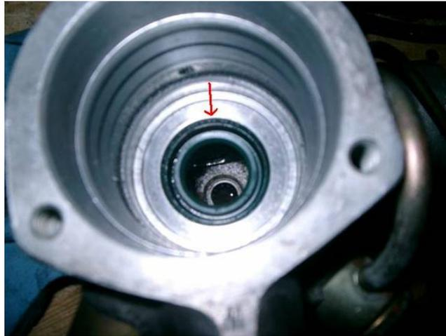
9. On the passenger side of the control tower, there is a large o ring in a groove that needs to be replaced. The smaller one you see actually came off the end of the shuttle, and belongs next to the white spacer that sits on the outside of the shuttle.
