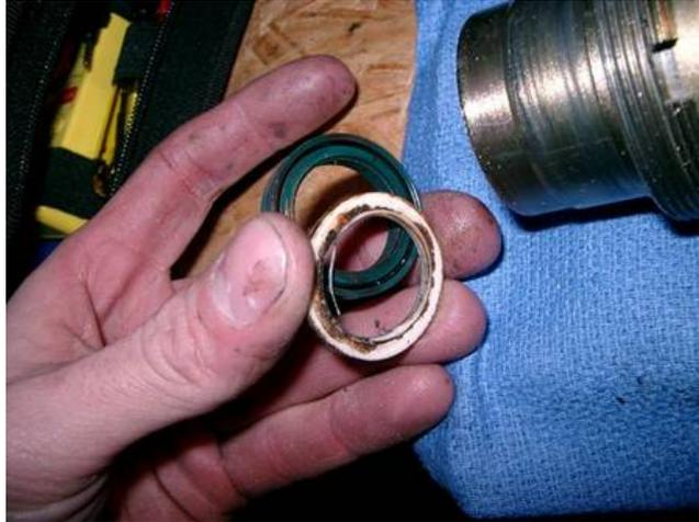
15. The above picture is misleading (not how it will come out of the sleeve), as the wiper seal is turned the wrong way, it should be flipped so that you are looking at the back of the seal (flat side).
