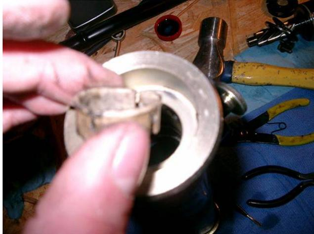
14. Next, take the appropriate size socket and knock out the wiper seal and spacer. Note, the tube size steps down as it gets closer to the seal, so if you put the tightest fitting socket in the end of the sleeve and try to pound out the seal, you will be hitting on the sleeve itself, and the seal won't move. I had use a socket that was a little smaller. The seal came out in about 3 hits.
