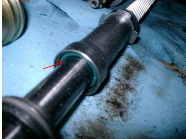
12. On the outside of the shuttle is a hard plastic ring, and a rubber o-ring that holds the ring onto the shaft. In the following picture, the plastic ring is on, but the o-ring is currently removed (it is actually seen in a previous picture if you read the description.) The o-ring will go on the outer side of the plastic ring (in the picture, to the right).
